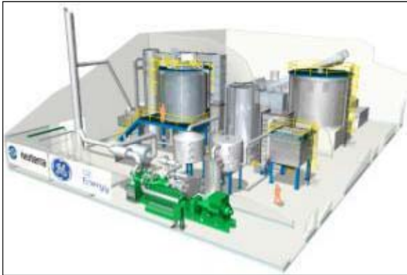
2 MW Nexterra biomass CHP plant
